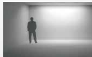
Wall washing Lighting
